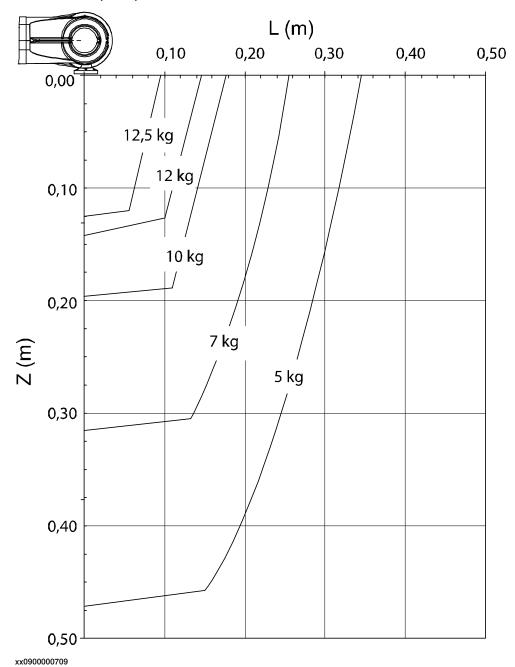
Extra load of 10 kg at the upper arm housing and 1 kg at wrist included in the load diagram.
