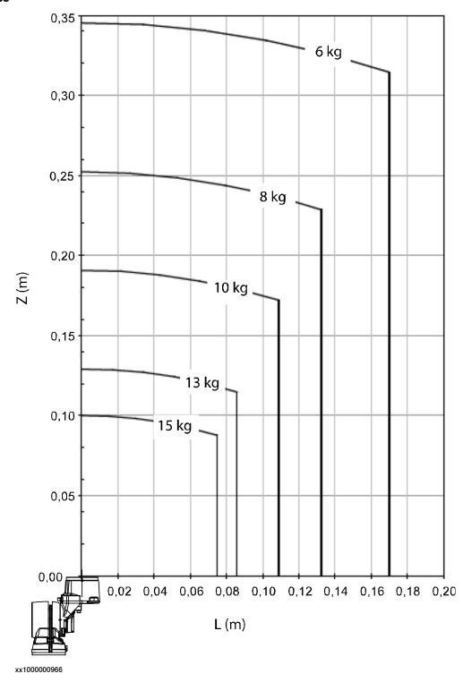
Extra load of 10 kg at upper arm and 1 kg at wrist included in the load diagram.
